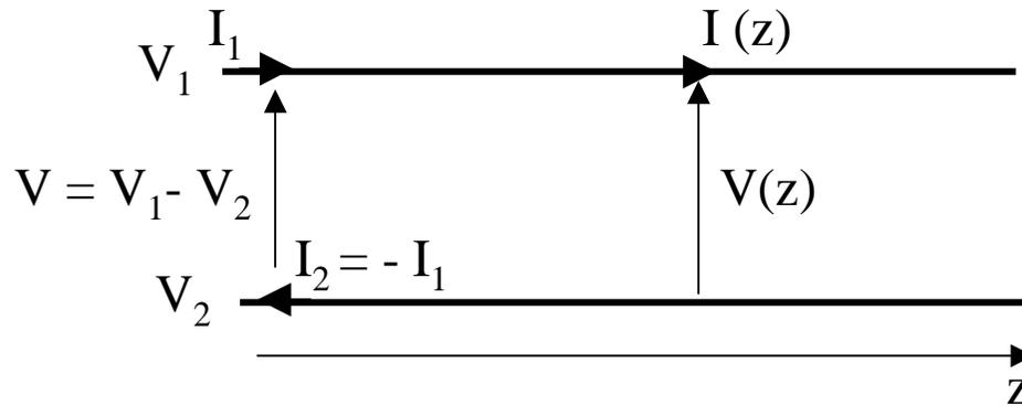
$$\frac{\partial V(z)}{\partial z} = -j\omega \frac{Z_c}{v} I(z) \quad (\text{éq.1})$$
