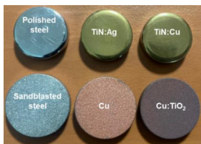
Figure 4: Photos of the PVD and PS samples elaborated and tested in this work.
